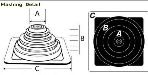
A= TOP OPENING DIMETER B= CUT TO SUIT PIPE SIZE C= BASE DIMENSIONS
