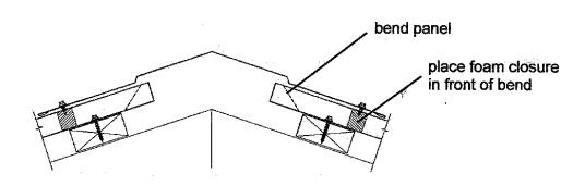
Notes: \*Turn Up Tool will bend roofing panels up to 24ga. thickness.
