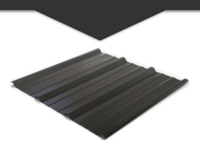
R-Panel/PBR-Panel is a low slope metal roof and wall panel with 1.25" high ribs at 12" apart. R-Panel installs quickly and cost efficiently on slopes as low as 1:12 making it our most popular panel chosen for commercial and agricultural use.
