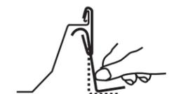
• With the upper clip firmly seated, position the base firmly against the purlin flange.
