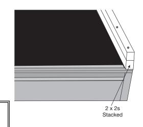
Pre-paint vertical/exposed portion of Villa Channel as needed prior to installing panels.
