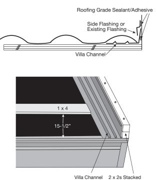
**Panels - First Course:** Fasten the first course of panels through the pre-punched fastening tabs to the 1 x 4s using minimum #9 Hex (1/4" diameter) x 1-1/2" long screws that will fit flush to panel and are long enough to penetrate the deck securely.
