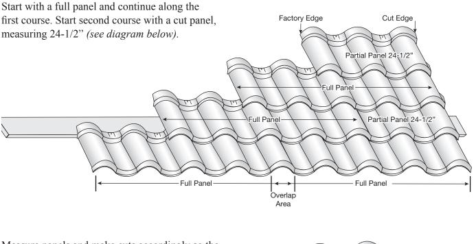
Measure panels and make cuts accordingly so the cut edge starts (or terminates) in the Villa Channel or Villa Valley *(see diagram below)*. Panels can be cut from either side *(see diagram right)*. Save cut-off pieces for use on opposite side terminating into Villa Valley or Villa Channel.
