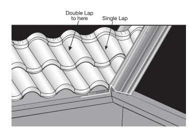
Pre-paint vertical/exposed portion of Villa Channel & Valley prior to installing panels.
