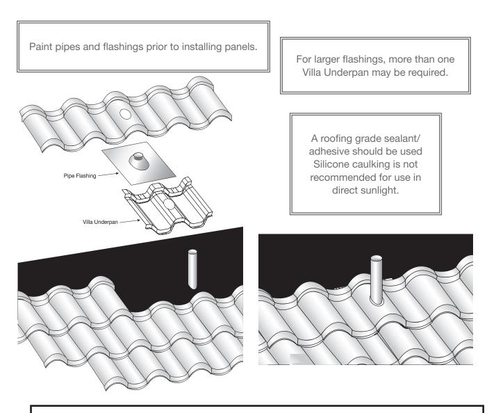
Do not use LEAD or COPPER with this steel roofing system.
