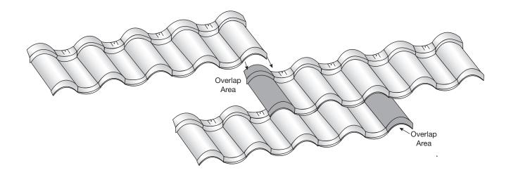
**Fastening Panels - Field:** Attach the second and subsequent courses of panels by locking the front of each panel into the back of the panel below. Fasten each panel to the deck with minimum #9 Hex (1/4" diameter) x 1-1/2" long corrosion resistant screws through the pre-punched fastening tabs along the back of the panels (*see diagram below*).
