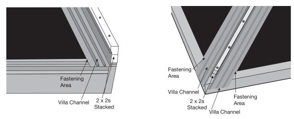
**Villa Valley:** Install Villa Valley or standard concrete valley metal (with same specifications as Villa Valley) along all valleys. All valley metal should be minimum 26 gauge pre-finished aluminum-zinc alloy coated steel. Valley metal should be a minimum 16" wide, with a minimum center upstand of 3-1/4". In new construction, the metal valley flashing must have one layer of Type 30 felt underlayment, 36" wide or ice & water shield underneath as required by local building code.
