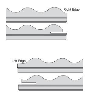
FASTENERS: (Villa Bird Stop - Eave) Minimum No. #9 Hex (1/4" diameter) x 1-1/2" Long Corrosion Resistant Screws (Color Coordinated)
