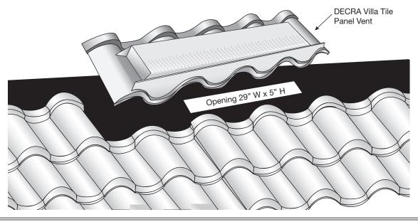
DECRA panel vents should be installed on the last full course below the ridge, and no more than 4 feet down from the peak of the roof facet. Panel vents should NOT be used for air intake.
