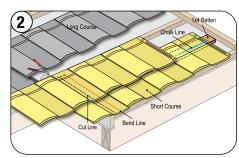
Place Long Course panel. Do not fasten. Properly align panels underneath to follow correct panel layout. Extend Short Course panel 1/2" (13 mm) past the eave. Mark the Bend Lines at the rake batten edge, and Cut Line, as shown. Mark the horizontal line on the Short Course panel aligned with the nose down-turn of the panel above. Install 1x4 Support Batten where two panel courses overlap.
