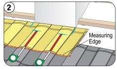
Align the front panel with the course below and the correct layout pattern for the profile, mark the sides of the chimney and mark the measurements from Step 1.
