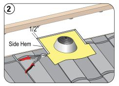
Place Pipe Jack on the panel to the side of the pipe and make 0.5" (13 mm) cuts in line with the back up-turn of the panel. Hem the edges, as shown.
