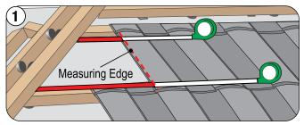
Measure and record the top and bottom of each hip cut (do this for the entire hip length on both the right & left side of the hip centerline). When measuring the hip panel cut, make sure to keep the tape measure in the same "plane" as the panels and parallel to the panel nose or back up-turn.
