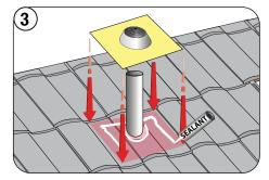
Apply bead of sealant to the panel. Position Pipe-Jack flashing over the pipe Press the Pipe-Jack flashing firmly over the contours of the panel.
