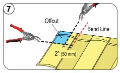
Add 2" to the left of Bend Line and mark as Cut Line. Cut and bend panel according to marked lines.
