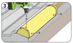
Fit the rake Starter Cap at the eave and fasten into the rake batten and into the side of the rake rafter, as shown.
