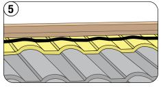
Place EmSeal Foam Tape (shown) or Foam Closure Strip at the top of the ridge cut.
