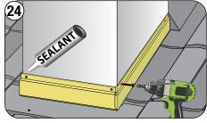
Complete Z-Bar installation up both sides, scribed to the Chimney saddle. Apply Sealant along the top edge of the Z-Bar.
