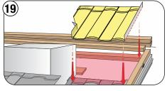
Install side panels on both sides, insuring they are sitting firmly on the back support batten.
