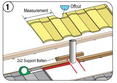
Install 2x2 support batten at the back of the pipe, minimum 12" (300 mm) long. Measure and cut lower panel to fit around the vent pipe. Install panel.
