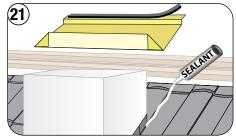
Apply Sealant down both sides of the panel in line with the chimney width. Apply an EmSeal tape to the back-flange of the Saddle.
