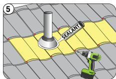
Install top panel and fasten as field panel. Apply sealant around the Pipe-Jack.
