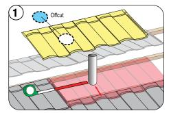
Measure, mark and cut the lower panel to fit around the vent pipe.
