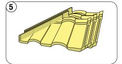
Stack each hip panel cut section in correct order, so they are easily accessible for installing in the correct spot on the roof.
