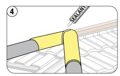
Apply a bead of sealant along the intersection.
