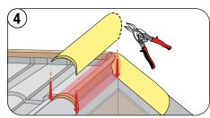
Fit each cap up the rake until it intersects with the ridge. Mark, cut and fit the final rake cap at the ridge.
