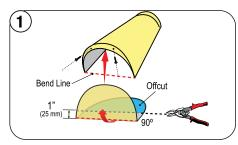
Insert the End Disk into Mission Cap and fasten with stitch screws. Bend End Disk at 90 degrees. Mark and cut to fit around the nose of the panel at the rake edge.
