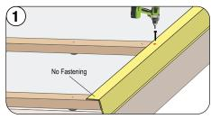
Install Fascia 3.5" metal up the rake. Fasten to each field batten. Do NOT fasten the Fascia 3.5" at the eave and rake corner until BirdStop is installed.
