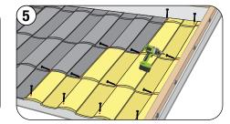
Fasten first rake cut through the back topflange. Fasten the following rake cuts in the same manner as full panels through the nose out of the main water channel and into the batten. Fasten rake cuts at the eave through the top into the eave batten.
