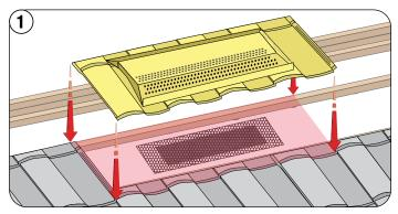
Cut a hole in the decking, approximately  $5" \times 30"$  (127 x 762 mm). Cover the hole with metal mesh (0.25" (6.5 mm) square) to prevent rodents from entering the attic.
