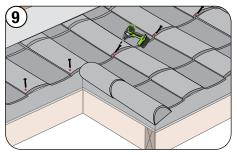
Finish installation of the Long Course and fasten as regular panels. Fasten through the top at the eave.
