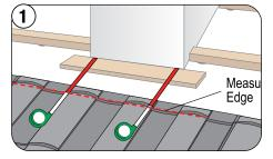
Install a support batten across the front and back of the Headwall/Chimney. Measure the front panel section as if it was a ridge cut panel. Deduct 1/2" (13 mm) from actual measurement to ensure an easy fit.
