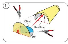
Insert the End Disk into Mission Cap and fasten with stitch screws. Bend End Disk at 90 degrees. Mark and cut at 45 degrees to fit around hip corner.
