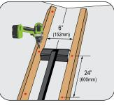
Valley Battens are spaced 6" apart to accommodate the Valley metal. Use Batten Spacer's 6" (152 mm) wide end to space the valley battens correctly and fasten at 24" o.c. (600 mm).
