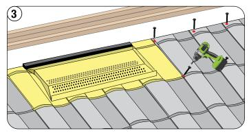
Continue installation of the panels in the row. Fasten as regular field panels.
