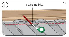
Measure the top row from the back-flange upstand to the ridge batten.
