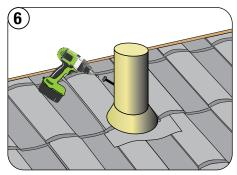
Install and fasten Pipe Sleeve from the back into the PVC pipe to finish the detail.
