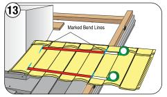
Align a full panel or panel section to the panel profile and mark the measurements.
