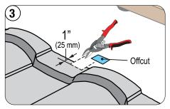
Notch the back top-flange of the panel 1" (25 mm) deep following the marked cut lines for the mount to fit over the panel.
