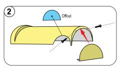
Cut out the rake cap profiles on each side and fit an end disc into the Ridge/Rake Starter Cap.
