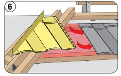
Install hip cuts starting from the top under the full panel.
