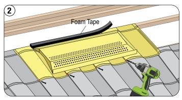
Install a section of EmSeal tape across the back edge where the ridge panel will overlap across the EZ-Vent. This provides additional weather protection across the back of the EZ-Vent. Fasten, as field panels.
