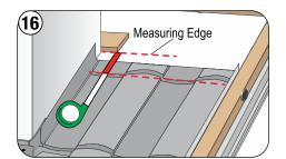
Measure from the Back-up Turn to the back of the chimney.
