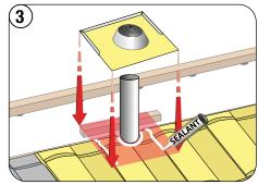
Apply sealant to the area where the Pipe-Jack will be installed.
