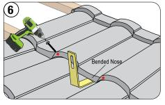
Install the panel above the Solar Roof Mount. Bend the panel nose where it intersects with the Solar Roof Mount to ensure a tight fit. Fasten the panel through the nose, as regular field panels.
