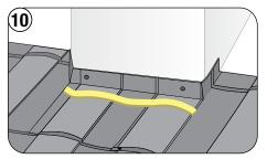
Place EmSeal tape or Foam Closure Strip across top of front panel section as a weather block.
