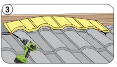
Fasten left end of the panel first, then right end, as shown.
