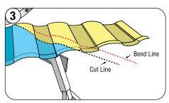
Using the Unified Steel<sup>®</sup> Cutter, start the cut from the nose edge of the panel to the back up-turn.
