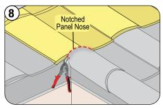
Install Long Course panel and notch the nose down-turn to fit Mission Cap.
