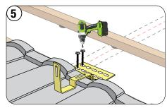
Install Solar Roof Mount with foot embedded in sealant and fasten with lag bolt screws, per local code.
