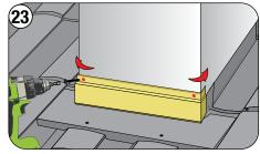
Measure, cut and bend Z-Bar metal, starting across the front.
