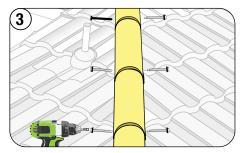
Fit each Mission Cap up the hip, making sure to keep the caps straight. Fasten through the sides into the hip batten, as shown.
