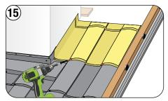
Install the side sections on both sides of the chimney and fasten as regular panels.
