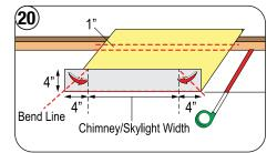
Using a section of Flat Sheet, mark and bend it up 4" (100 mm) minimum, forming a saddle flashing for the back of the item being flashed. Make sure it is 4" (100 mm) wider on each side of Chimney/Skylight.
