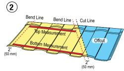
Apply top and bottom measurement to a full panel. Add 2" (50 mm) to allow bend-up.
