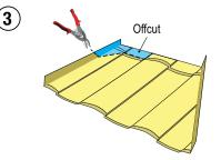
The top left corner needs to be cut and flattened to fit under the valley exit area.
