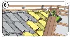
Fasten the following valley cuts in the same manner as full panels through the nose **out of the main water channel** and into the batten.
