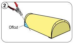
Notch inside corner of the first Starter Cap, as shown, to allow it to fit on the bottom panel course.
