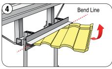
Using the Unified Steel<sup>®</sup> Bender, insert the hip cut into the bender jaws, clamping the hip cut section and bend the hip section up to create an approximate 1.5" to 2" (38 to 50 mm) bend up on the panel section.
