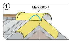
Position the Ridge/Rake Starter Cap as shown and scribe the profile of the rake caps on either side.
