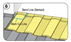
Place marked panel to the side of the chimney, align with the front panel and mark Cut Line, aligned with the Chimney/ Skylight front edge.
