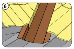
The rest of the panels above are measured, marked, cut and bent and fitted as regular hip or valley panels cut sections.
