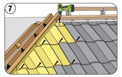
Fasten first hip cut through the back topflange. Fasten the following hip cuts in the same manner as full panels through the nose **out of the main water channel** and into the batten.
