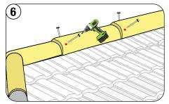
Continue Installing Mission Caps on the ridge. Fasten with 2 fasteners, one on each side, into the ridge batten.
