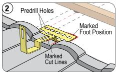
Place the mount over the pan section of the back top-flange. Adjust the foot of the mount so the holes of the foot are aligned with the center of the rafter. Predrill the holes and mark the width of the bridge touching the panel and projected foot location.
