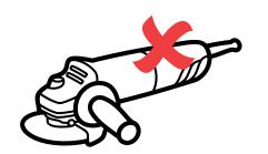
Circular saw or grinder wheel to cut panels is NOT acceptable.
