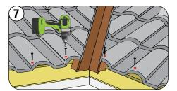
Fasten the course across the eave through the top of the panel out of the main water channel, behind the BirdStop upturn.
