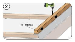
Place 2x2 EBS batten on top of Fascia 3.5" and keep 2x2 pads flush with the rake edge. Fasten into each field panel batten, except the eave batten.
