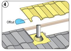
Install full panel to the side of the pipe. Mark the top panel to where the flashing cone base will align, cut out this piece to allow the panel to fit around the flashing cone.
