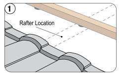
Lift up upper Unified Steel roof panel. Find and mark the location of the rafter beneath the roof deck.
