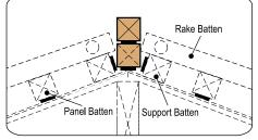
Ridge battens can be positioned side by side, or vertically stacked as shown, using 2x2 EBS battens or 2x2 battens.
