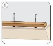
Position the first Eave Batten so the top corner of the batten is in line with the fascia. Fasten through the batten and plastic pad into the wood deck.
