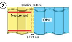
Apply measurements to the full panel and mark the Bend Line. Add 1.5" (38 mm) and mark the Cut Line.
