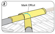
Position the ridge cap over the intersecting hip caps and scribe the hip cap profiles on both sides.
