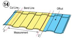
Apply Bend Line measurements to the panel. Add 2" to mark Cut Line.
