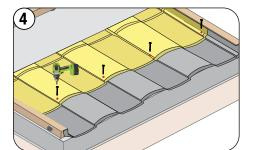
Install panel above the Short Course eave panel. Fasten through the top into EmSeal foam tape.
