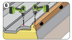
Fasten rake batten at the eave/ rake corner AFTER you have aligned the BirdStop flashing with the panel profile.
