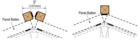
Hip battens can be positioned side by side, or vertically stacked as shown, using 2x2 EBS battens or 2x2 battens.
