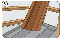
Install the Valley Open 6" metal seating it down into the sealant.
