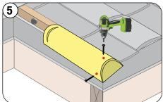
Form and install Mission Cap Starter (End Cap) and fasten through the top into the rake batten and on the side, as shown.
