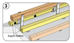
Place support battens (shown in yellow) across the ridge. Support battens allow the ridge cut bent panel to be seated in the same roof plane as the rest of the field.
