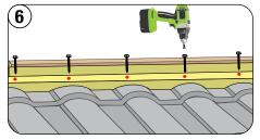
Install Top Row metal and fasten trough the top flange, as shown.
