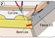
At the eave and rake intersection, the BirdStop is cut and folded **UNDER** the Fascia 3.5" metal.
