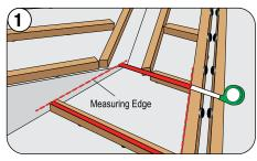
Measure the top and bottom of the panel section from the side wall to the hip batten.
