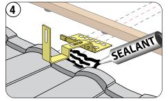
Apply a bead of sealant beneath Solar Roof Mount foot and in each predrilled hole before placing it into position.
