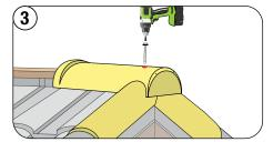
Fasten the Ridge/Rake Starter Cap through the top into the ridge batten.
