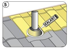
Apply sealant around the cone.
