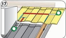
Align a full panel or panel section to the panel profile. Apply the previous measurement and mark as Cut Line. Measure the distance from the Chimney/ Skylight to the Rake batten and make as Bend Line.
