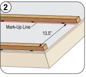
Measure 13.5" (343 mm) from the front eave /fascia batten to the batten above. Use a string line to position the second batten to allow adequate overhang at the fascia for gutter/water shed from the roof.
