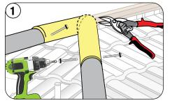
Position the two hip caps at the ridge intersection. Mark and cut them to fit by overlapping each other. Fasten, as shown.
