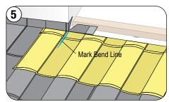
Align side panel with the course below and the correct layout pattern for the profile and mark the Bend Line aligned with the Chimney/Skylight side edge.
