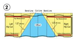
Apply measurements to the full panel and mark the Bend Line. Add 1.5" (38 mm) or use 2x2 batten and mark the Cut Line on the other side.
