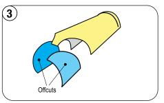
Cut out the ridge cap scribed lines to fit over the two intersecting hip caps.
