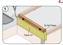
Install Fascia 3.5" and 2x2 Batten at the Short Course rake. Do not fasten at the rake/eave corner.
