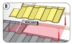
Apply Sealant and fit the side panel aligning it with the field panels already installed.
