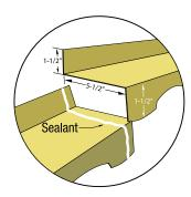
Overlap Top Row 2" (50 mm). Apply a bead of Sealant between two overlapping Top Row pieces.
