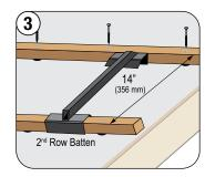
Working across and up the roof, position the Batten Spacer over the second row batten. Position the next batten firmly against the top face of the Batten Spacer and fasten. Pay careful attention to positioning the batten spacer the correct way.
