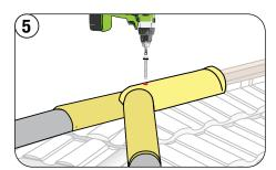
Fit the ridge cap and fasten into the ridge batten. Use the Touch-Up kit to seal fasteners.
