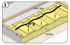
Add 1.5" (38 mm) to the marked Bend Lines and mark as Cut Lines. Cut and bend panels. Install the Short Course panel. Install BirdStop at the eave. Finish the row. Fasten panel through the top at the eave. Apply EmSeal foam tape just above the marked chalk line.
