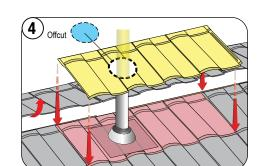
Measure, mark and cut the top cover panel around the cone base to fit around the flashing cone.
