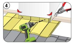
Fit the front bottom flashing section as shown and cut at a 45 degree angle from each side, bend the corners around the Headwall/Chimney.
