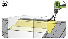
Fasten each end of the Saddle through the back-flange under EmSeal tape.
