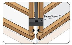
Install hip battens 5" (125 mm) apart. Use the Batten Spacer's small flange for this spacing. Rotate EBS batten so the plastic pads are facing towards the hip center line. Fasten at each batten intersection.
