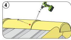
Install ridge Mission Caps and fasten on both sides into the ridge batten, as shown.
