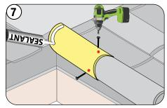
Fasten Mission Cap cut into the rake batten and on the side. Apply a bead of Sealant on top, as shown.
