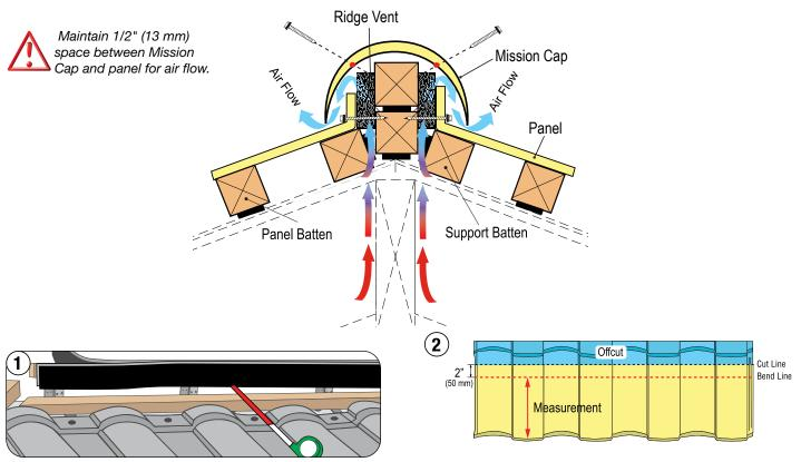
Measure the top row from the Back-Flange upstand to the Ridge Vent material.
