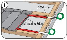
Measure and record the top and bottom of each panel cut.
