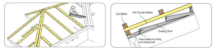
Position 1x4 Counter Batten over rafter, maximum 24" o.c. Fasteners must penetrate 1" (25 mm) into or through the roof framing members and be placed 12" (305 mm) o.c. Consult local codes for all re-roofing requirements.
