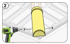
Fasten the Starter Cap through the sides.
