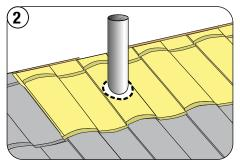
Install lower panel to fit around the vent pipe.
