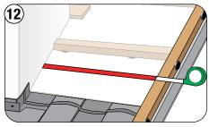
Measure the distance from the side of the Chimney to the rake batten.
