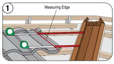
Measure and record the top and bottom of each panel cut. Keep the tape measure in the same "plane" as the panels and parallel to the panel nose or back up-turn.
