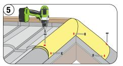
Fasten at the top and sides. Use the Touch-Up kit to finish this detail.
