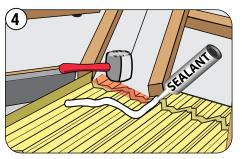
Install the valley exit panel to fit under the dormer eave overhang and valley exit. Apply Sealant to the valley exit area.
