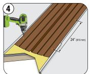
Insert Valley Five 'V' into the Valley Exit. Fasten Valley with washer and grommet screws in the outside locations a minimum of 24" o.c. (610 mm) up both sides.
