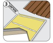
Fit the Exit Tray at the fascia. Apply Sealant, as shown.
