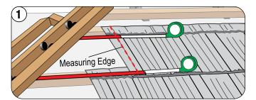
Measure and record the top and bottom of each hip cut (do this for the entire hip length on both the right & left side of the hip centerline). When measuring the hip panel cut, make sure to keep the tape measure in the same "plane" as the panels and parallel to the panel nose or back up-turn.
