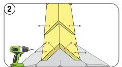
Form the ridge Starter Shake Cap, fit and fasten, as shown. Continue installing caps at the ridge, fastening with 2 screws to the ridge batten on both sides.
