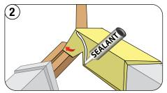
Cut and fit the Shake Cap section. Bend the left end slightly. Apply Sealant along the center line.
