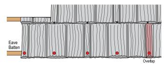
Fasten the bottom row panels through the top of the panel on the left or the right side of each concave section, out of the main water channel of the panel. **NOTE:** Top panel fastening is also acceptable behind EZ-Vents and Chimney/Skylight details, as necessary.
