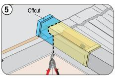
Place next Shake Cap on top of the Starter Cap at the corner intersection. Mark and cut, as shown.
