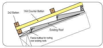
Position 1x4 Counter Batten over rafter, maximum 24" o.c. Fasteners must penetrate 1" (25 mm) into or through the roof framing members and be placed 12" (305 mm) o.c. Consult local codes for all re-roofing requirements.
