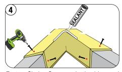
Fasten Shake Caps on both sides and apply Sealant at the top of intersected Shake Caps.
