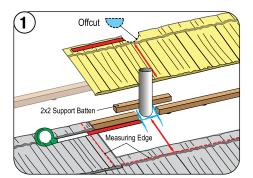
Measure and cut lower panel to fit around the vent pipe. Install panel.
