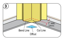
Cut the valley exit point and bend to form an internal corner.
