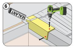
Fasten Shake Cap cut into the rake batten and on the side. Apply a bead of Sealant on top, as shown.
