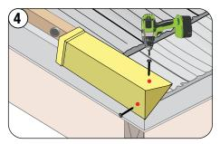
Form and install Shake Cap Starter (End Cap) and fasten through the top into the rake batten and on the side, as shown.
