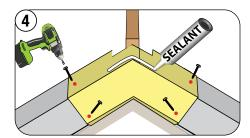
Fit the left Shake Cap. Overlap at the top and fasten, as shown.
