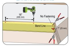
Place Fascia 3.5" metal at the eave and extend 1" (25 mm) over the rake/gable edge. Cut and bend to fit around the corner, as shown. Fasten through the top flange 16" (406 mm) o.c. DO NOT fasten at the intersection with rake.
