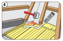
Install the valley exit panel to fit under the dormer eave overhang and valley exit. Flatten back flange against the roof deck and apply Sealant, as shown.
