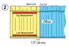
Apply measurements to the full panel and mark the Bend Line. Add 1.5" (38 mm) or use 2x2 batten and mark the Cut line.
