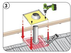
Slide the Pipe-Jack flashing over the pipe and seat it into the Sealant. Press firmly. Fasten the front side of the Pipe-Jack flashing with Stitch Screws, as shown.
