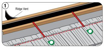
Position Ridge Vent on both sides of ridge batten. Measure the top row from the back-flange upstand to the Ridge Vent material.
