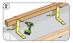
Place a 2x2 wood nailer board into Ridge Riser Brackets. Fasten wood nailer to Ridge Riser Brackets with a #8 min. 0.75" (19 mm) screw or roofing nail.
