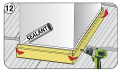
Complete Z-Bar installation up both sides bending at the corners. Apply Sealant along the top edge of the Z-Bar.
