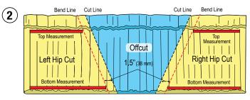
Apply measurements to the full panel and mark as Bend Line. Add 1.5" (38 mm) or use 2x2 batten and mark the Cut Line on the other side.
