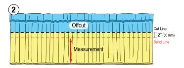
Apply measurements to the full panel. Mark Bend Line, add 2" (50 mm) and mark a Cut Line. Bend up and cut ridge panel.
