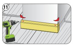
Measure, cut and bend Z-Bar metal, starting across the front. Fasten, as shown
