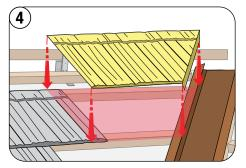
Install the valley cut sections in the same manner as full panels. Start at the ridge and work down to the eave.
