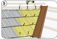
Fasten first valley cut through the back top-flange. Fasten the following valley cuts in the same manner as full panels through the nose out of the main water channel and into the batten. Fasten hip cuts at the eave through the top into the eave batten.
