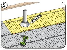
Install top panel and fasten as field panel. Apply Sealant and granules around the Pipe-Jack.
