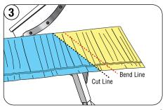
Cut the panel using the Unified Steel® Cutter.
