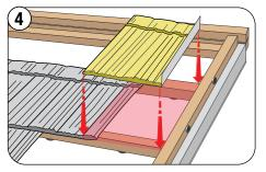
Install rake cut panels from the ridge down to the eave.
