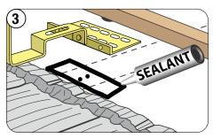
Apply a bead of Sealant beneath Solar Roof Mount foot and in each predrilled hole before placing it into position.
