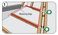
Measure the top and bottom of the panel section from the side wall to the hip batten.
