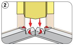
Cut and bend Fascia 3.5, as shown. Slide the Valley Open 6" into position. Extend Valley a minimum of 1" (25 mm) past the bend section of the Fascia 3.5".
