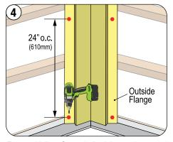
Fasten Valley Open "6" with regular panel fasteners on both outside flanges at 24" o.c. (610 mm).
