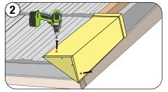
Position the rake Starter Cap at the fascia at 90 degree. Fasten into the rake batten and into the side of the Shake Cap, as shown
