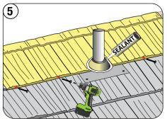
Fasten panel as regular field panel. Apply Sealant and stone chip around the flashing cone
