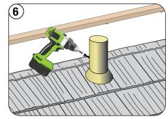
Install and fasten the Pipe-Sleeve through the back of the sleeve into the pipe. Make sure to fasten at least 2" (50 mm) above the Pipe-Jack cone.
