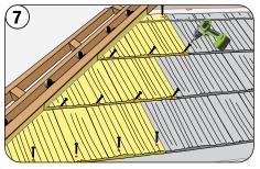
Fasten first hip cut through the back topflange. Fasten the following hip cuts in the same manner as full panels through the nose **out of the main water channel** and into the batten. Fasten hip cuts at the eave through the top into the eave batten.
