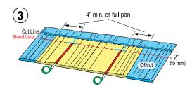
Apply the measurements to a full panel and bend the entire length then cut off the excess.
