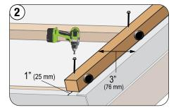
Install 2x2 EBS Batten 3" (76 mm) from the rake edge and 1" (25 mm) from the eave and fasten into each field batten.
