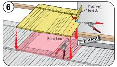
Cut and bend up the panel, as shown. Bend the corner around Chimney/ Skylight. Apply Sealant and fit the left-side panel aligning it with the field panels already installed.
