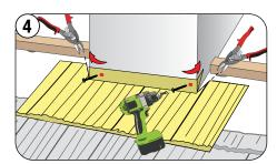
Fit the front bottom flashing section and cut at a 45 degree angle from each side. Bend the corners around the Chimney/ Skylight. Fasten with 2 screws, as shown.
