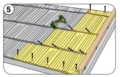
Fasten first rake cut through the back topflange. Fasten the following rake cuts in the same manner as full panels through the nose **out of the main water channel** and into the batten. Fasten rake cuts at the eave through the top into the eave batten.
