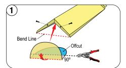
Insert the End Disk into Trim Cap and fasten with Stitch Screws. Bend End Disk at 90 degrees. Add 1/2" (13 mm) to the Bend Line. Mark and cut to fit around the nose of the panel at the rake edge.
