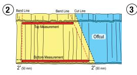
Apply measurements to a full panel. Add 2" (38 mm) to allow bend-up.
