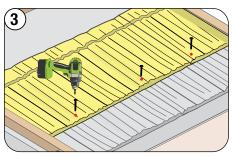
Install panel above the Short Course eave panel. Fasten through the top into EmSeal foam tape and 1x4 support batten.
