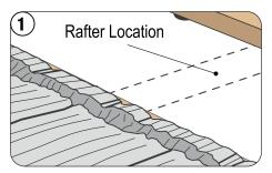
Lift up upper Unified Steel roof panel. Find and mark the location of the rafter beneath the roof deck.
