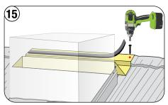
Fasten each end of the Saddle through the back-top flange. Apply an EmSeal tape on the Saddle aligned with the backtop flange of the panels.
