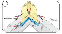
Place top Shake Cap on the ridge 2" (50 mm) beyond the edge. Mark the Bend Line along the edge. Add 1" (25 mm) and mark the Cut Line. Notch at the intersection with the hip caps below.
