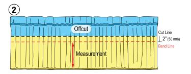
Apply measurements to the full panel. Mark Bend Line, add 2" (50 mm) and mark a Cut Line. Bend up and cut ridge panel.
