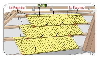
Panel layout starts at the top full course of panels in any roof section. Panels are laid from the **ridge down to the fascia**. Position first full panel on the top panel batten 24" (600 mm) maximum from the rake batten, as shown.
