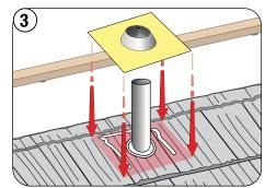
Slide the Pipe-Jack flashing over the pipe and seat it into the Sealant. Press firmly.
