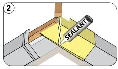
Fit the Shake cap and apply Sealant to the center line.
