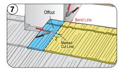
Align the right-side panel with the Chimney/ Skylight and panel below keeping correct layout pattern. Mark the Bend Line. Add 2" (50 mm) to the Bend Line and mark the Cut Line. Mark the distance from the panel nose to the front of the Chimney/ Skylight and mark horizontal cut.
