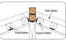
Ridge battens can be positioned side by side, or vertically stacked as shown, using 2x2 EBS battens or 2x2 battens.
