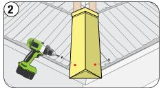
Fit Starter Shake Cap and fasten through the sides into the hip battens.
