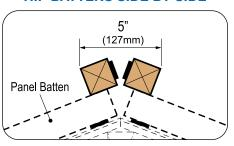
Hip battens can be positioned side by side, or vertically stacked as shown, using 2x2 EBS battens or 2x2 battens.
