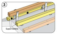
Place support battens (shown in yellow) across the ridge. Support battens allow the ridge cut bent panel to be seated in the same roof plane as the rest of the field.
