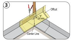
Place the left Shake Cap on top and mark the Cut Lines along the center line. Add 1" (25 mm) at the top for overlap.
