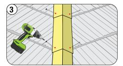
Fit each Shake Cap up the hip, making sure to keep the caps straight. Fasten through the sides into the batten.
