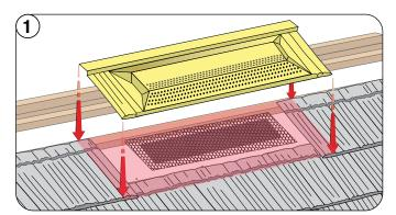
Cut a hole in the decking, approximately 5"  $\times$  30" (127  $\times$  762 mm). Cover the hole with metal mesh (0.25" (6.5 mm) square) to prevent pests from entering the attic.
