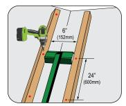
Valley Battens are spaced 6" apart to accommodate the Valley metal. Use Batten Spacer's 6" (152 mm) wide end to space the valley battens correctly and fasten at 24" o.c. (600 mm).
