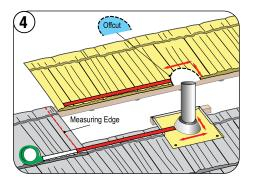
Install full panel to the side of the pipe. Mark the top panel to where the flashing cone base will align, cut out this piece to allow the panel to fit around the flashing cone.
