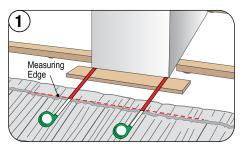
Install a support batten across the front and back of the Chimney/Skylight. Measure the front panel section as if it was a ridge cut panel. Deduct 1/2" (13 mm) from actual measurement to ensure an easy fit.
