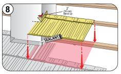
Cut and bend up panel. Apply Sealant to the corner and down the panel. Bend the corner of the bend-up and fit the panel.
