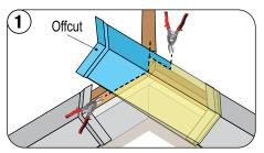
At the ridge intersection, place right Shake Cap and mark Cut Lines, as shown.
