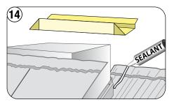
Apply Sealant down both sides of the panel in line with the Chimney/Skylight width.
