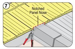
Install Long Course panel and notch the nose down-turn to fit Shake Cap.
