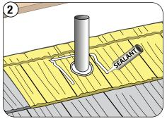
Install base panel to fit around the vent pipe. Apply a bead of Sealant on each side and around the hole of the pipe, as shown.
