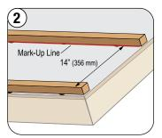
Measure 14" (356 mm) from the front eave /fascia batten to the batten above. Use a string line to position the second batten to allow adequate overhang at the fascia for gutter/water shed from the roof.
