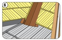
The rest of the panels above are measured, marked, cut and bent and fitted as regular hip or valley panels cut sections.
