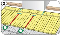
Align the front panel with the course below and the correct layout pattern for the profile, mark the sides of the chimney and mark the measurements from step 1.
