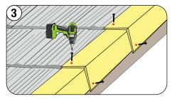
Fit each Shake Cap up the rake. Fasten each cap with 2 fasteners, as shown.
