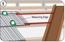
Measure and record the top and bottom of each panel cut, as shown. Keep the tape measure in the same "plane" as the panels and parallel to the panel nose or back up-turn.
