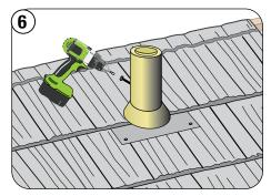
Install Pipe Sleeve and fasten from the back into the PVC pipe to finish the detail.
