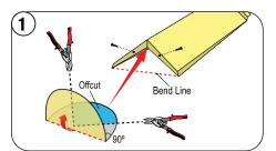
Insert the End Disk into Trim Shake Cap and fasten with stitch screws. Bend End Disk at 90 degrees. Mark and cut at 45 degrees to fit around hip corner.
