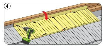
Push panel down to fit coursing properly. Force back of panel into position against ridge batten. Continue fastening ridge cut panel across the nose. Next, fasten panel through bendup into ridge batten.
