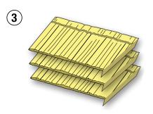
Cut and bend panels. Stack each valley cut section in correct order, so they are easily accessible for installing in the correct spot on the roof.
