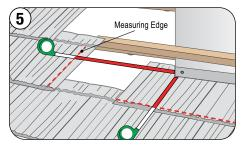
Measure the distance from the panel overlap to the Chimney/Skylight and mark on the left-side panel as a Bend Line. Add 2" (50 mm) and mark as a Cut Line.
