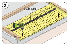
Add 1.5" (38 mm) to the marked Bend Lines and mark as Cut Lines. Cut and bend panels. Install the Short Course panel and extend it 1/2" (13 mm) past the eave. Finish the row. Fasten as regular eave panels. Apply EmSeal foam tape above the marked chalk line.
