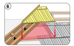
Install hip cuts starting from the ridge and work down to the eave.
