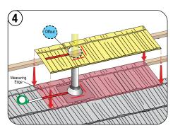
Measure, mark and cut the top cover panel around the cone base to fit around the flashing cone.
