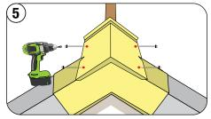
Install first ridge cap, aligning starting edge with rake caps. Fasten into ridge battens.
