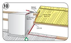
Align the top panel to the course below. Measure the distance from the back flange to the back of the Chimney/Skylight and mark Cut Line, as shown. Install panel section and apply Sealant across top edge of the bend-up.
