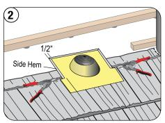
Place Pipe Jack on the panel to the side of the pipe and make 1/2" (13 mm) cuts in line with the back up-turn of the panel. Hem the edges, as shown.
