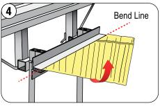
Using the Unified Steel® Bender, insert the hip cut into the bender jaws, clamping the hip cut section and bend the hip section up to create an approximate 1.5" to 2" (38 to 50 mm) bend up on the panel section.
