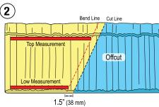
Apply measurements to the full panel and mark the Bend Line. Add 1.5" (38 mm) and mark the Cut Line on the other side.
