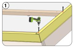
Install Fascia 3.5" metal up the rake. Fasten into each field batten
