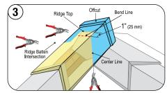
Place other Shake Cap on top. Mark the Bend Line at the ridge top and Cut Line along the center line. Add 1" (25 mm) to the Bend Line and mark as Cut Line. Notch the back side up the ridge batten.
