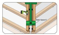
Install hip battens 5" (125 mm) apart. Use the PINE-CREST Shake Batten Spacer's small flange for this spacing. Rotate EBS batten so the plastic pads are facing towards the hip center line. Fasten at each batten intersection.
