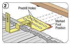
Place the mount over the back top-flange. Adjust the foot of the mount so the holes of the foot are aligned with the center of the rafter. Predrill the holes and mark the projected foot position.
