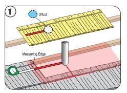
Measure, mark and cut a pipe sized hole in the base panel.
