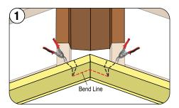
Notch the Fascia 3.5", as shown, to allow the valley pan to exit. Extend Valley 1" (25 mm) minimum past fascia.
