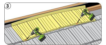
Align ridge panel with the panel below. Fasten left end of the panel first, then right end.
