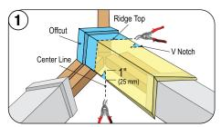
Place the Shake Cap at the ridge intersection. Mark the Cut Line at the ridge top and V-notch the right side at the point of the ridge battens, and left side at the center line. Cut, as shown
